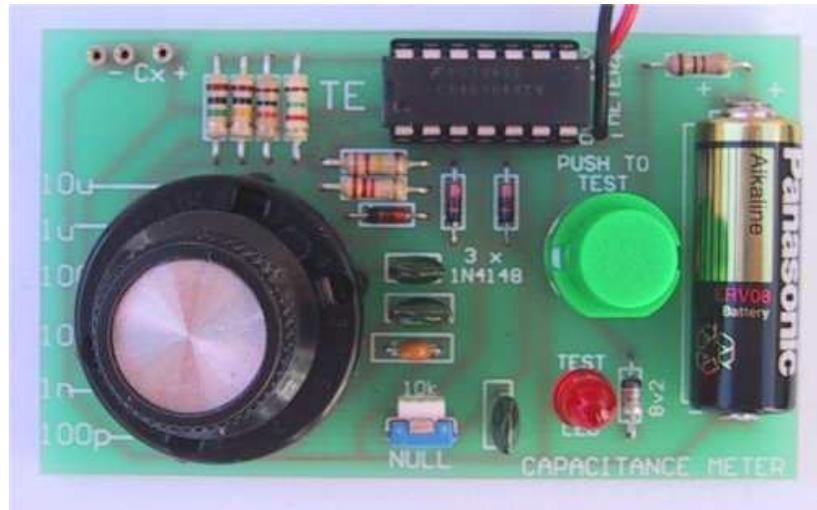
Figure 3.6: The Add-on Capacitance Meter by Mitchel, C.
