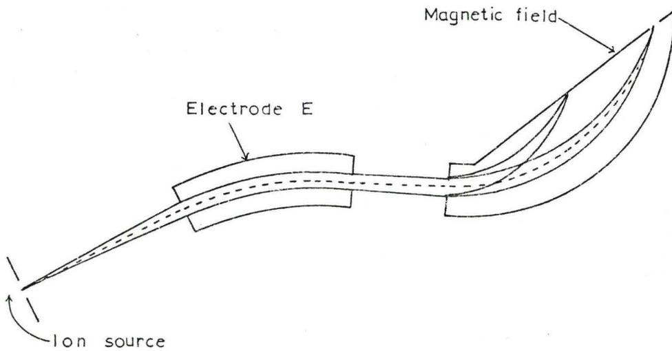
Figure 2. Double focusing design of Mattauch and Herzog
